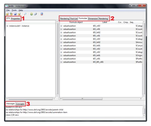
In the area marked with "Number 1", there will be two tabs: DTS and Properties views. DTS offers an expandable tree view of the document DTS.
