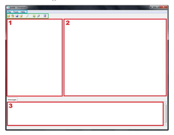
The window is divided in various sections, as seen in the picture above. Marked with a blue rectangle, right below the Toolbar, there is the Menubar, and marked with red rectangles and divided into three sections, there is the main workspace.
