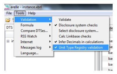
This screen will allow you to select the specific checks that the validation process will carry out.
